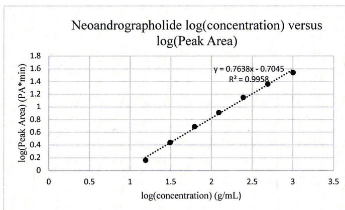
Figure 8: Calibration Curve for Neoandrographolide.
