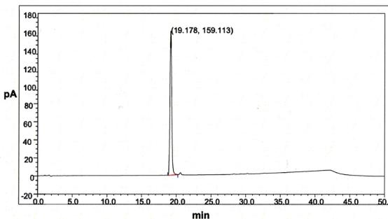
Figure 3: HPLC Results for Neoandrographolide Standard (1 mg/mL).
